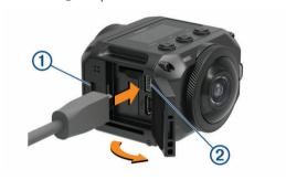
2 Plug the cable into the VIDEO port 2 on the camera.
